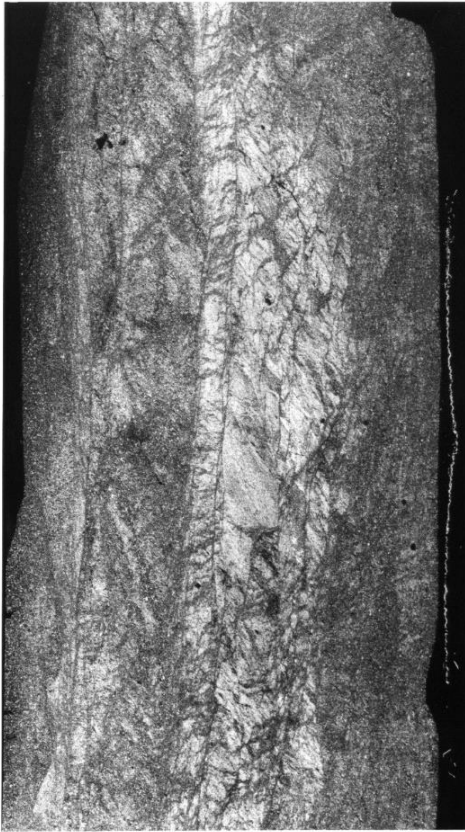
Figure 27. Thin section specimen, \approx 10\text{mm} wide, showing well-developed (vertical) principal displacement shears, from ICP pile shaft shear zone in silty Pentre clay, after Chow (1997).
